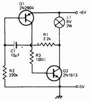
This simple circuit will flash a 6 volt lamp at a rate determined by the size of capacitor C1. It is most economical on power as it only draws current when the lamp is ON. When the lamp is OFF both transistors are biased OFF.
